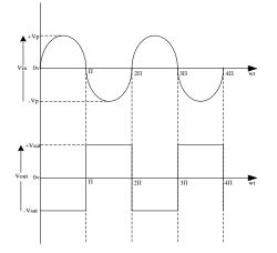
Figure 6: Waveforms of ZCD
