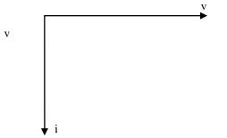
Figure 3: Phasor diagram for purely inductive load.
